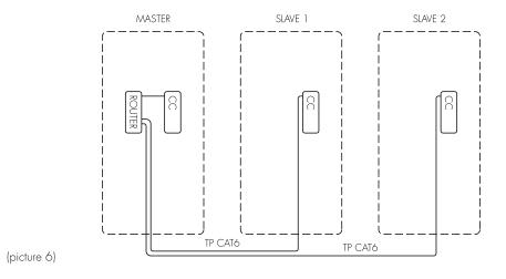
5pcs LS4 connected with TP CAT6 cable to router/switch
